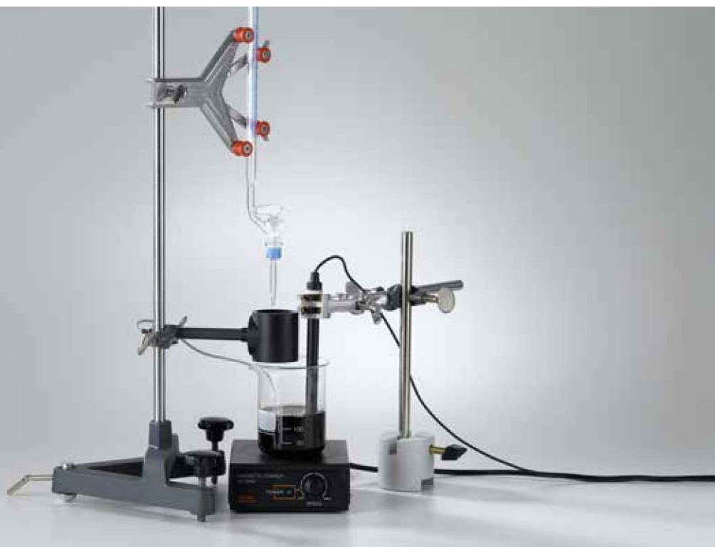
Determination of acid concentration by titration with drop counter (C3.5.1.1)
